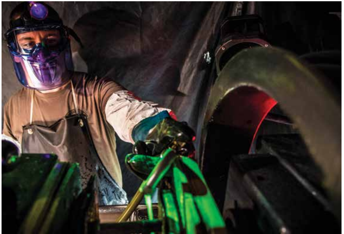
U.S. Air Force Tech. Sgt. Eric Suarez, nondestructive inspection noncommissioned officer in charge, 108th Maintenance Squadron, analyzes a KC-135R Stratotanker part, Sept. 22, 2019. The process involves magnetizing the part, which is then bathed in a suspended particle bath that seeps into the defects and when exposed to ultraviolet light – black light, causes the defects to become florescent and visible.
